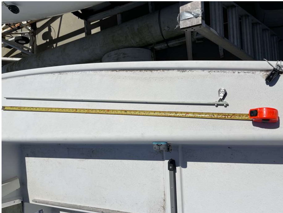
The 4'6" mast whip with bullet block installed.
