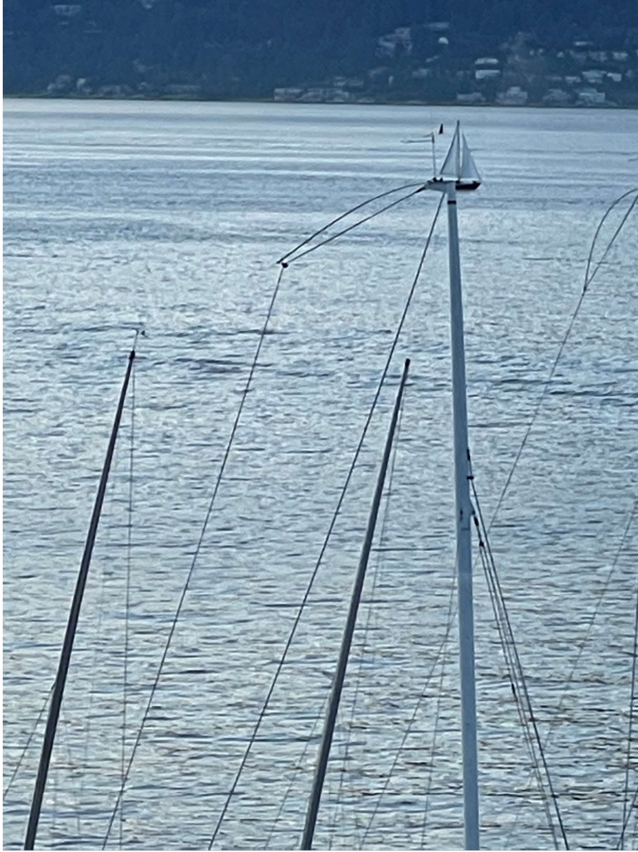
The extra-long mast whip as seen from the upper deck at RVYC using a zoom lens. Note how far aft the backstay line is projected.
