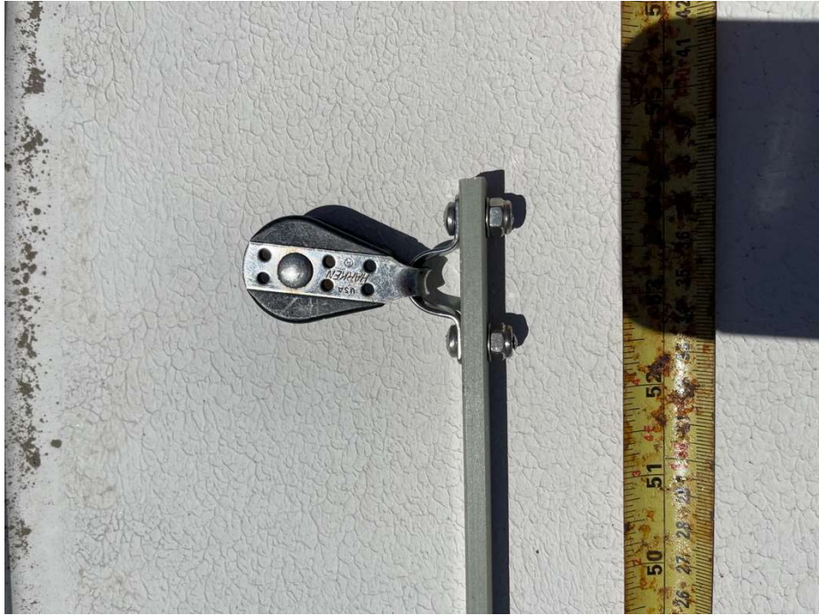
Eyestrapping bolted on to mast whip aft end.
