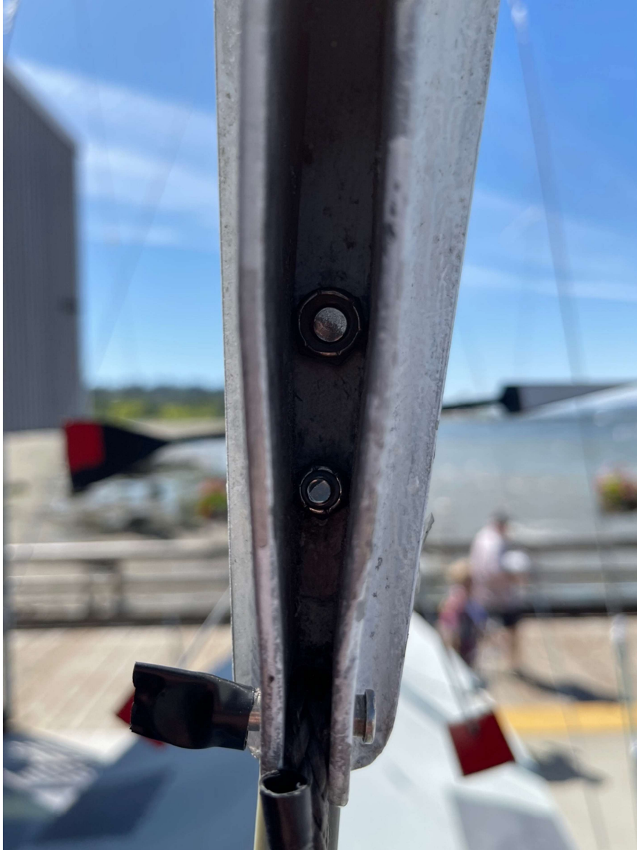
Under-view of the mast crane with two of the nuts holding the mast whip in place. The aft screw is not visible.
